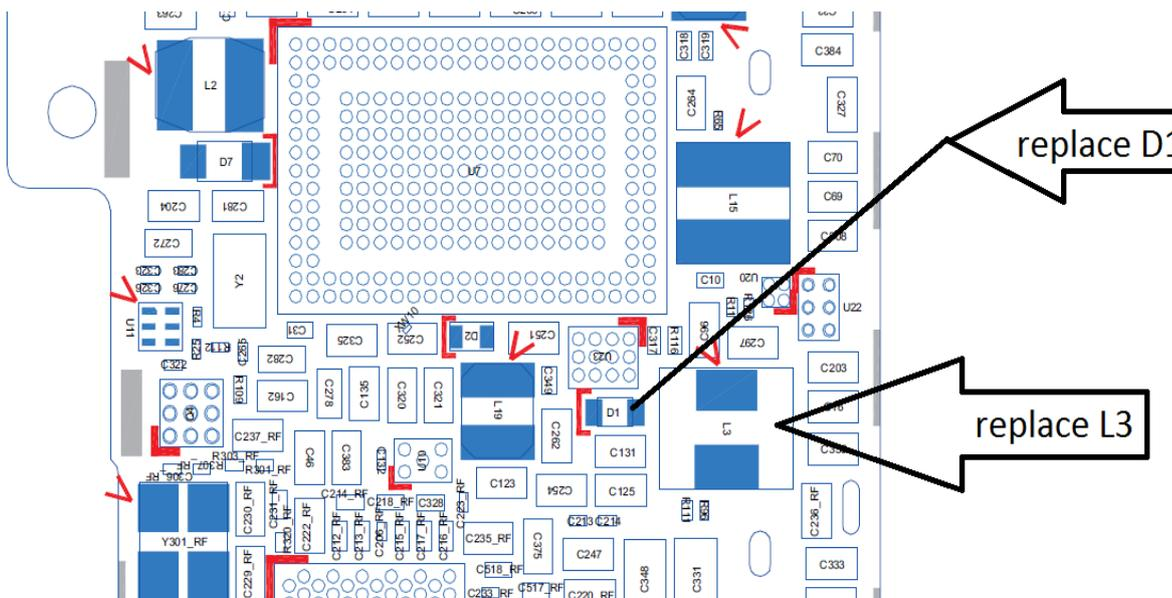
This repair should not be attempted by anyone without the necessary soldering experience It is supplied only to provide the location details of the components in the supplied kit **computabench** will not be held responsible for any damage caused by the incorrect fitting of the parts or incorrect temperatures used therein please note that these parts should not be fitted until a correct diagnosis has first been completed to determine their failure
