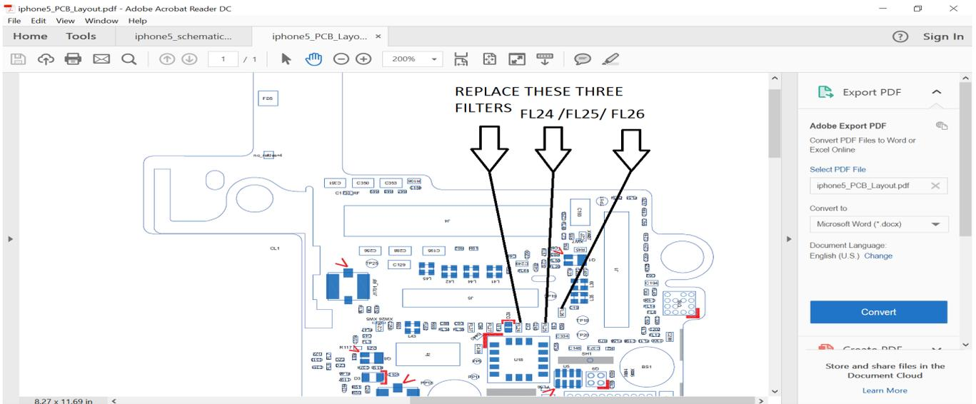
remove the PRINTED CIRCUIT BOARD and change the above three filters with the ones included in the kit next turn the pcb over and locate the components **IN THE DIAGRAM BELOW** note the correct orientation of the diode (D1) the cathode or marked end of the diode is indicated by the red line at the left of the component the replacement must be fitted in the same direction.
